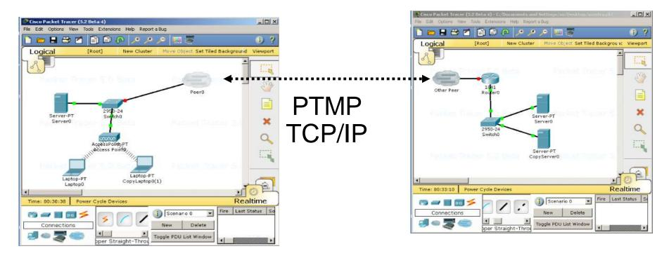
The Multiuser connection (Peer0 in the picture) can connect by TCP/IP to a Multiuser connection of another PT (Instance on a different computer)
