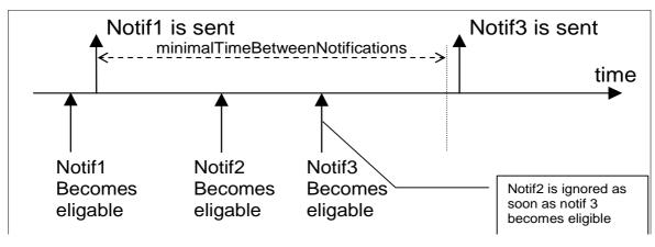
Figure 9.82: Notification mechanism when minimalTimeBetweenNotifications is used, the case when more than one notification become eligible
