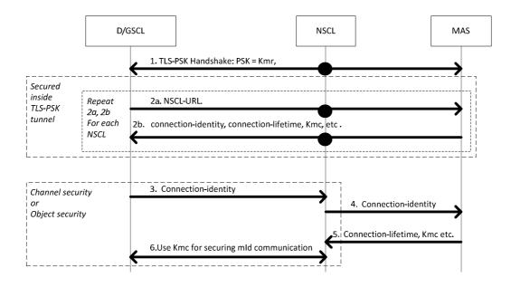
Figure 8.12: High Level Call flow for M2M Service Connection procedure based on TLS-PSK when using object security or channel security for mld Data Security
