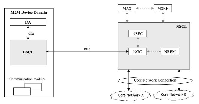
Figure 8.1: Functional architecture elements for automated bootstrapping
