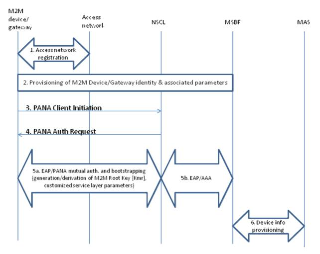
Figure 8.6: M2M Service Bootstrap using automated method
