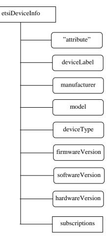
Figure B.6: Structure of the etsiDeviceInfo resource
