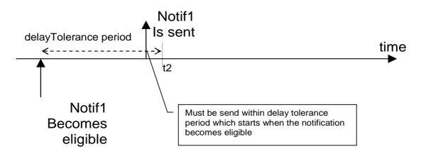
Figure 9.83: Notification mechanism when delayTolerance is used
