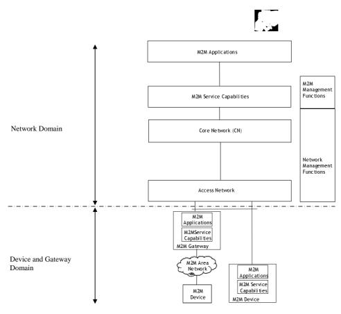
Figure 4.1: High level architecture for M2M
