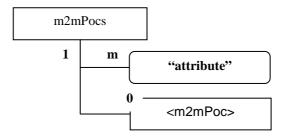
Figure 9.24: Structure of m2mPocs resource
