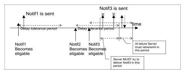
Figure 9.85: Notification mechanism, the case of failure to transmit notifications on time
