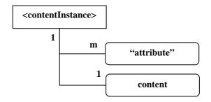
Figure 9.17: Structure of <contentInstance> resource
