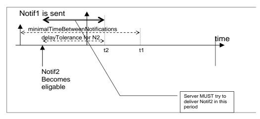
Figure 9.87: Notification mechanism, conflict between the subscription minimalTimeBetweenNotification and the resource instance delayTolerance
