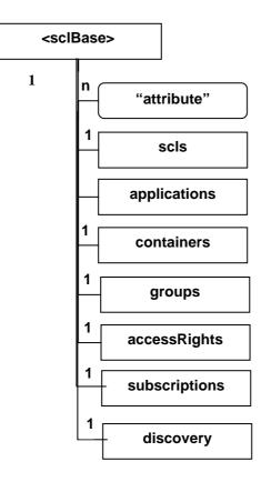
Figure 9.2: Structure of <sclBase>-resources
