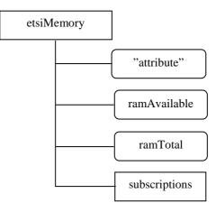
Figure B.12: Structure of the etsiMemory resource
