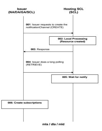
Figure 9.113: Procedures for <notificationChannel> create
