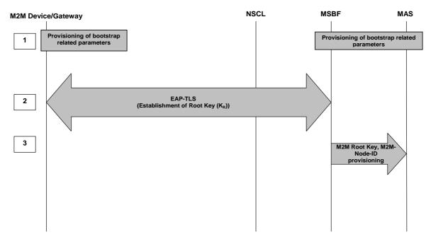
Figure 8.8: M2M Service Bootstrap using EAP-TLS over PANA
