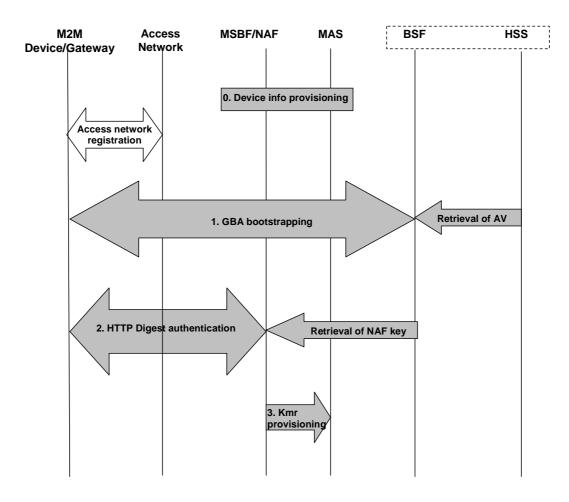
Figure 8.4: M2M Service Bootstrap based on GBA
