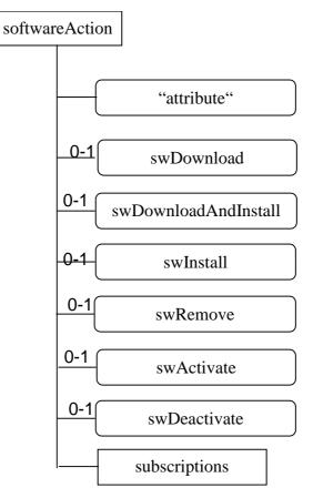
Figure B.23: Structure of the softwareAction resource
