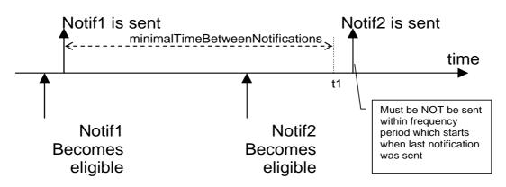
Figure 9.81: Notification mechanism when minimalTimeBetweenNotifications is used
