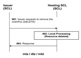
Figure 9.93: Procedures for <m2mPoc> delete
