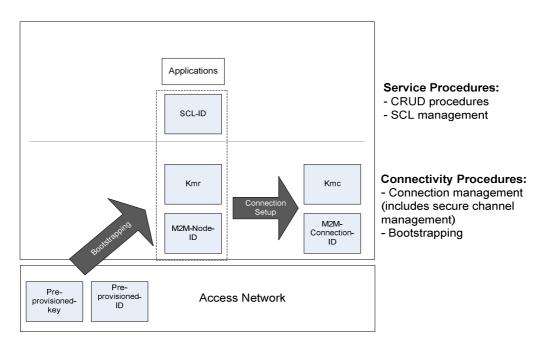
Figure 7.2: M2M identifiers provisioning overview when M2M bootstrap is performed through leveraging access network credentials
