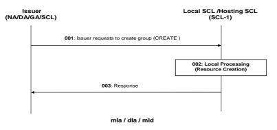
Figure 9.71: Illustration of Procedures to Create Group
