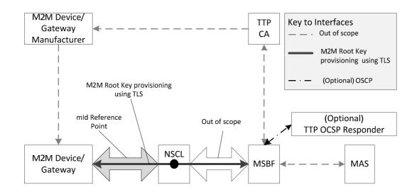
NOTE: The line through the NSCL indicates that the NSCL passes messages between D/G M2M Node and MSBF with some procedure-dependent processing at NSCL.
