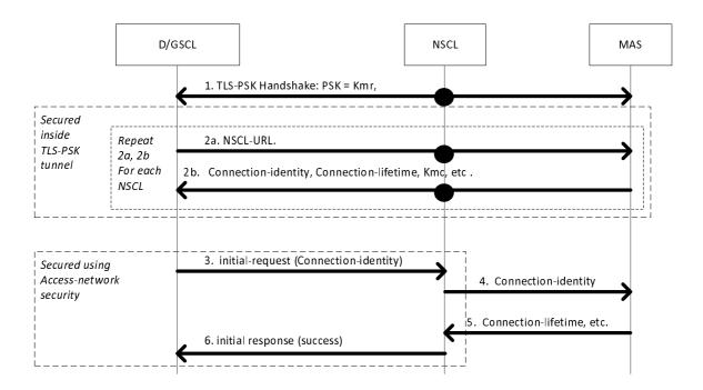
Figure 8.13: High Level Call flow for M2M Service Connection procedure based on TLS-PSK when using access network security for mld Data Security
