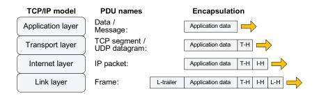
An example of TCP/IP encapsulation
