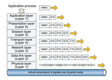
And each layer in the destination system analyzes and removes this control information
