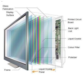
The typical multi-layered structure of an active-matrix liquid crystal display
