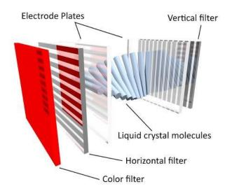
A subpixel of a colour LCD display. The crystal cells are arranged in a twisted spiral form due to the twisted nematic effect
